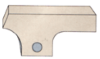
Thick sections in Connection to thin sections can cause contraction. Therefore design the part to leave sufficient allowance to machining.
