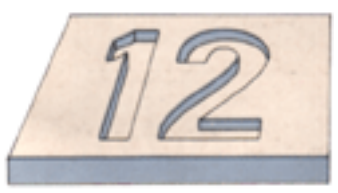
Text can be cast in parts, than raised leters.
